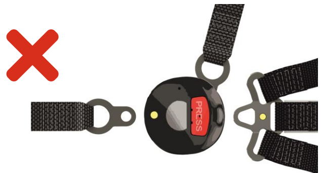
this figure shows the wrong installation of the left 5 Point Net Buckle System 09077
